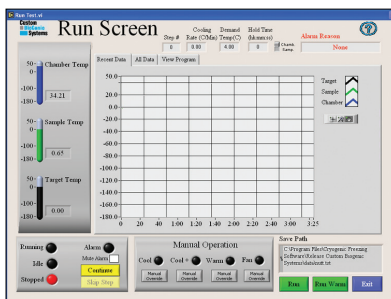
Run screen provides all details of actual freeze runs during operation, plus all manual override controls.
